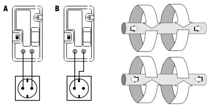
This effect is eliminated by separating the current paths. While one socket is connected to the line to be tested, the return line should not lie within the same cable or cable channel. One solution is to connect the return line to a separate ground, for example central heating, a water pipe or a sprinkler system. The other solution is to connect it to a remote outlet via a cable reel.
