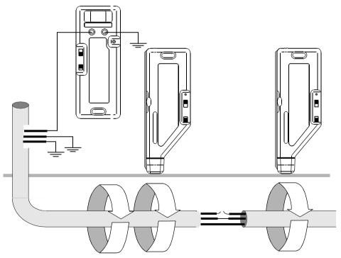
Even in the case of a broken cable, a sufficient signal current for location of the line normally flows through the soil here. If, however, no current flow takes place, it is also possible to measured in the *open circuit mode*.
